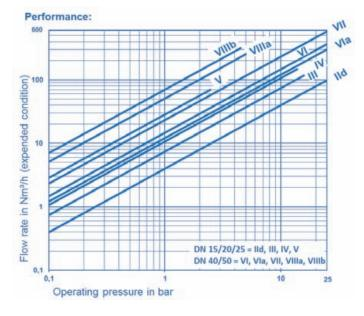
The performance diagram applies to venting into atmosphere, i. e. without back pressure. The performance values apply to normal air expansion. The performance value of air being under pressure is determined by dividing the value of the diagram by operating pressure in bar.
