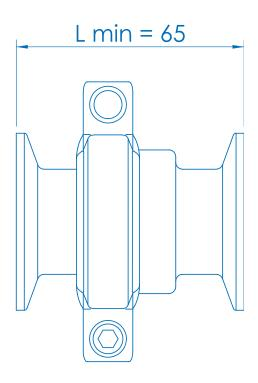
The installation dimension can be extended on request.
